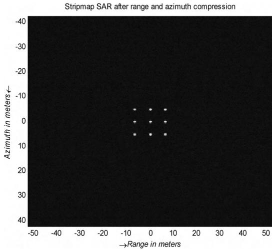
Figure 7 Image result of Point array target
