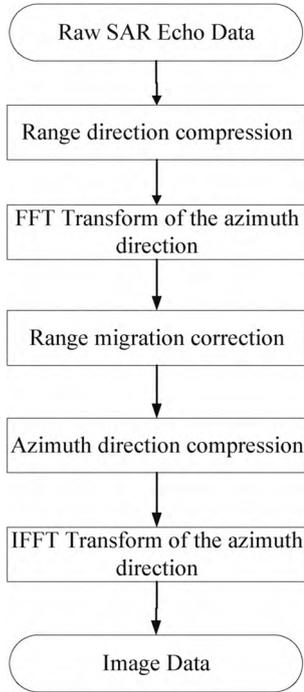
Figure 4 Block diagram of RD algorithm
